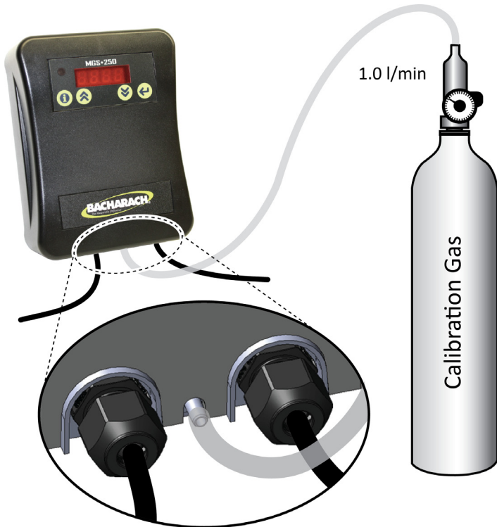
Figure 16. Using Calibration Gas
